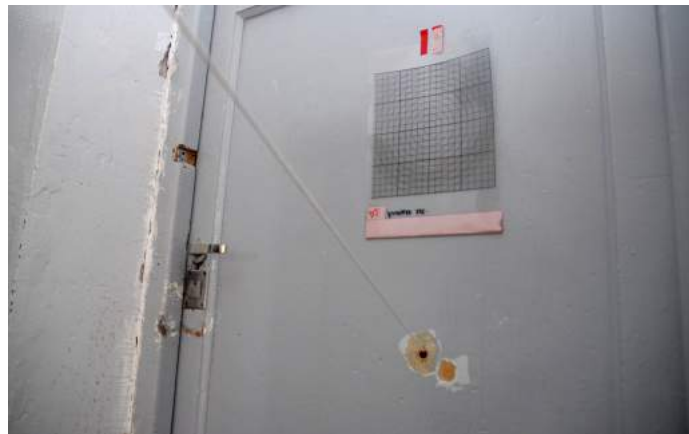
Figure 36 The uncovered orifice in the door. The string indicates the central direction of the cone of possible directions of the shot.
